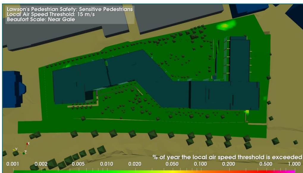
Figure 60: Sensitive Pedestrian Safety Criterion: View of the entire site
